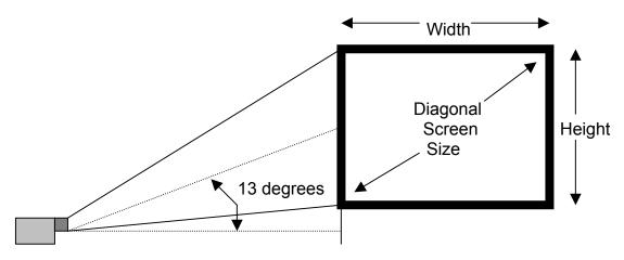
Use the following information to position the projector. Horizontally the projector needs to be positions with the lens-centered left to right
